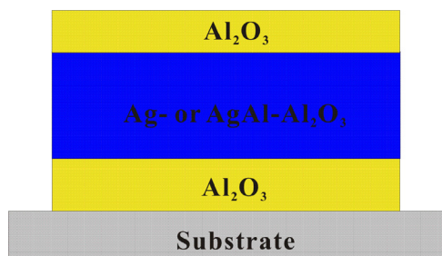
Fig. 1. Schematic diagram of the sandwich structure for thermal stability investigations.
