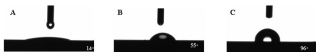
Fig. 2 Static water contact angle measurements for (A) silicon wafer treated by fresh piranha solution. (B) Patterned \text{Py-CH}_2\text{NH}_2 active surface on the silicon substrate. (C) Polystyrene brushes grafted from the patterned \text{Py-CH}_2\text{NH}_2 coated silicon substrate.
