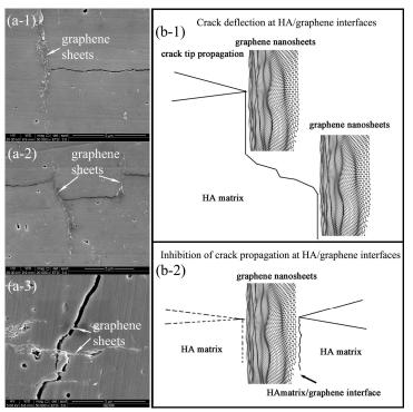
Figure 5. Inhibition of crack propagation by graphene nano-sheets in the SPS HA-rGO composites. (a) FESEM images showing termination of the crack growth by graphene nano-sheets at the crack tip (a-1), deflection of the crack attained by graphene nano-sheets (a-2) and bridging of the crack by graphene nano-sheets (a-3). The corresponding regimes are schematically illustrated in the right panels (b-1,2).
