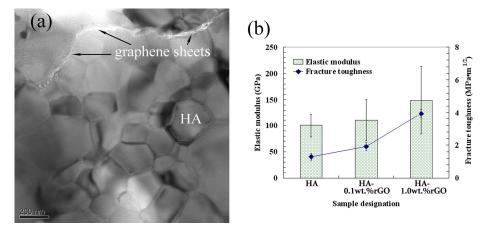
Figure 4. TEM image showing intact graphene nano-sheets in the SPS HA-rGO pellets (a), and the addition of rGO significantly improved fracture toughness and elastic modulus of the SPS HA-rGO pellets (b).
