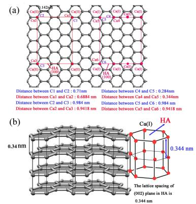
Figure 3. Schematic illustration of the matched atomic arrangement at (a) the interface between the planes (300) and (100) of HA and graphene surface, and (b) the interface between the (002) plane of HA and cross-section of graphene sheets.
