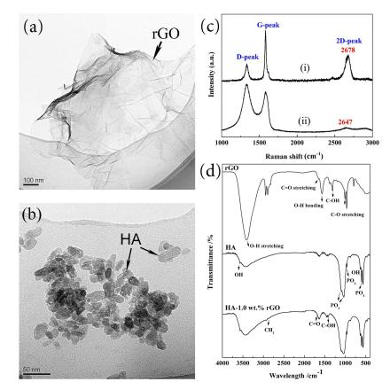
Figure 1. TEM images and structure analyses of the synthesized rGO and HA-rGO composites,
