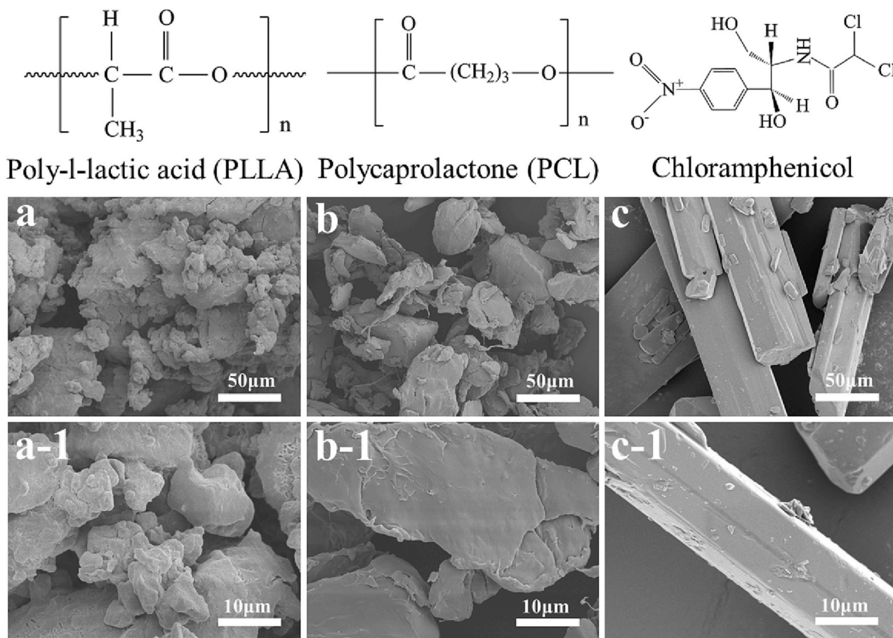
Fig. 1. Depiction of the chemical structure and SEM images of the polymers and drug employed in this study, the corresponding magnified SEM images are shown as (–1). (a, a-1) PLLA powder, (b, b-1) PCL powder, and (c, c-1) CAM powder.
